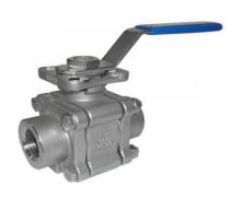
AUTOMA 3-piece body is full bore design with straight through flow. 3piece body allows easy maintenance service without removing end cap from pipe line. The body is made of investment casting and the valve is featured with blow-out-proof stem. Suitable for isolation applications in the Food Industries, Palm Oil and Refinery, Rubber Glove, Power, Oil and Gas, Petrochemical Industries and Genral Industrial Plants.
